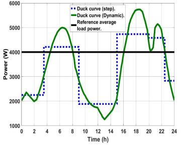
Fig. 4. Formation of duck curve by adding solar.
