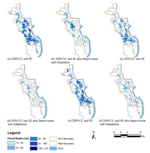
Fig. 12. (a) Waterlogging scenario for 2020 under climate change and sea level rise (b) Waterlogging scenario for 2020 under climate change and sea level rise with improvement and adaptation
