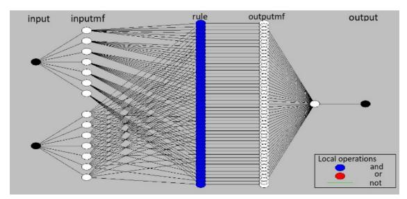
Fig. 14. ANFIS structure showing input(s) and output.
