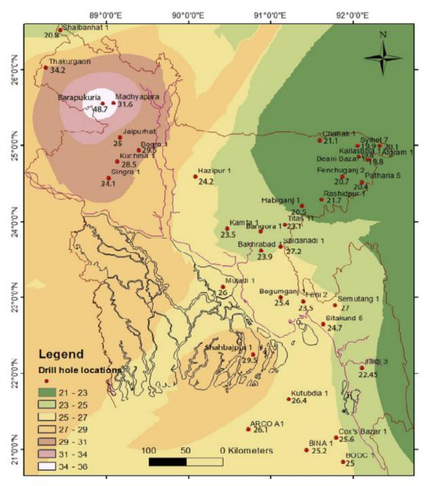
Fig. 5. Well wise temperature gradient of Bangladesh. (Source: [37])
