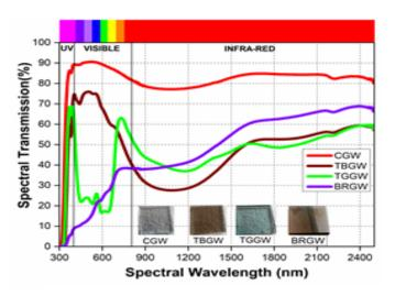
Fig. 3. Spectral transmission of glass materials.
