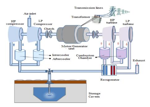
Fig. 12. Compressed air storage system [16].
