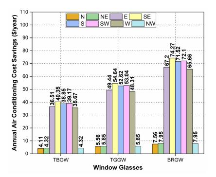
Fig. 7. Annual air conditioning cost savings of buildings using various glass windows compare with a clear glass window.
