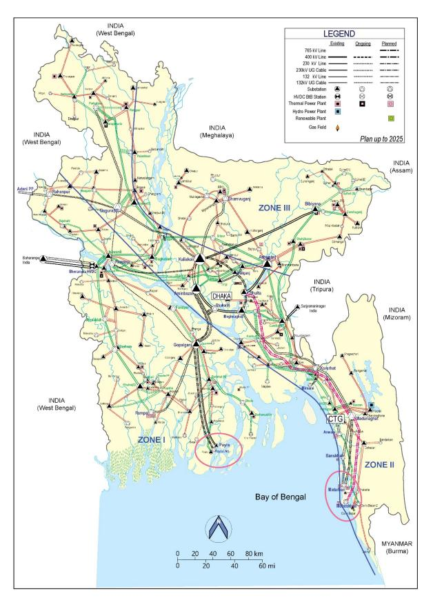
Fig. 3. Map of the Power Grid Plan 2020-25 of Bangladesh [67]. The three earthquake zones are marked (solid blue lines) on top of the map to show the spatial distribution of the power grid infrastructures. Red ellipses mark the three under construction power hubs [65] in which in Matarbari and Maheskhali located in the south-east, and Payra is located southwest of the map.
