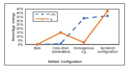
Fig. 4. Optical absorption enhancement (g) and short-circuit current density (J<sub>sc</sub>) comparison between different nanostructure configurations with respect to that of bare Silicon substrate [12].
