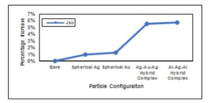
Fig. 9. Percentage change comparison for short-circuit current density (J<sub>sc</sub>) for different nanoparticle configurations [13].
