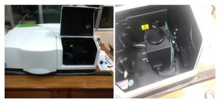
Fig. 2. UV-Vis-NIR Perkin Elmer (Lambda 950) spectrophotometer.
