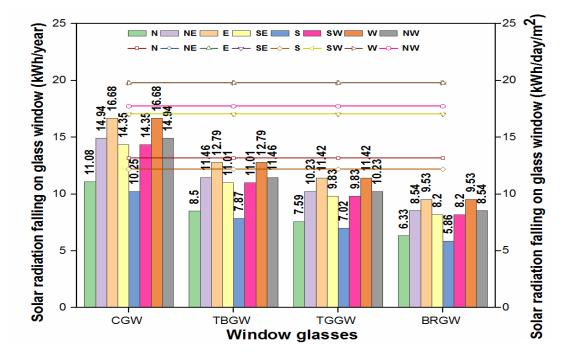
Fig. 5. Solar radiation falling and passing through window glazing of the Dhaka region on a peak summer day.
