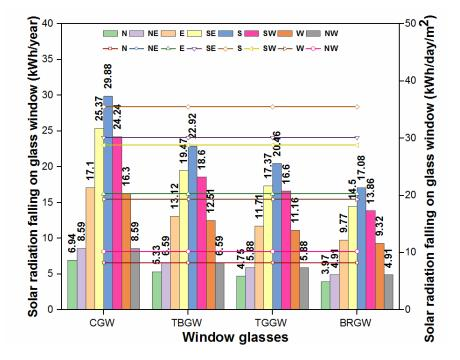
Fig. 6. Solar radiation falling and passing through window glazing of the Dhaka region on a peak winter day.
