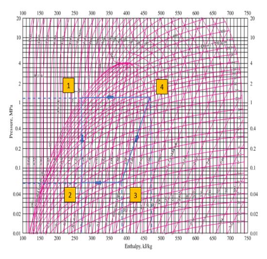
Fig. 7. Presure versus enthalpy diagram for refrigerant R134a.
