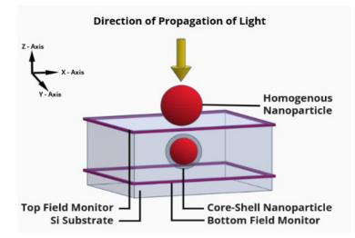
Fig. 3. Simulation setup showing frequency domain field and power monitor placements for "sandwich" configuration of homogenous NP and core-shell NP coupled to a solar cell.
