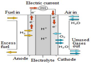
Fig. 18. Basic structure of fuel cell system [28].
