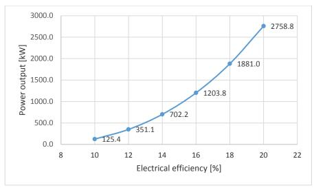
Fig. 2. Power output as function of electrical efficiency.
