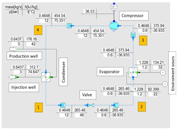
Fig. 6. IPSEpro simulation model.
