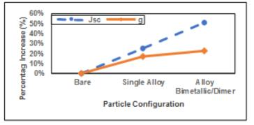
Fig. 7. Percentage change comparison for optical absorption enhancement factor (g) and short circuit current density (J<sub>sc</sub>) for different nanoparticle configurations [14].
